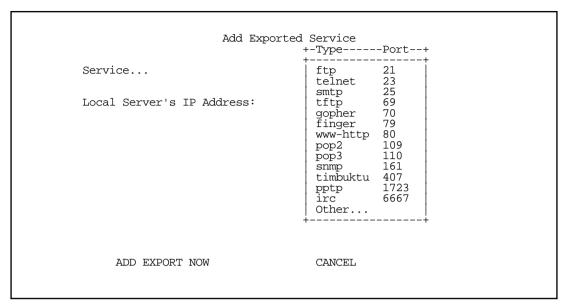
8. Select any of the services/ports and press Return to associate it with the address of a server on your local area network. For example, if you select **www-http 80**, press Return, and type **10.0.0.2**, the Netopia R5000 Series Router redirects any incoming traffic destined for a Web server to address 10.0.0.2.
